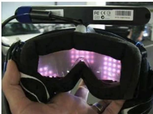
We began by showing nearby objects as bright regions of light. We made a test system using a depth camera and an array of LEDs and attached a pair of ski goggles. As you see in this video, that's enough information for you to infer that there is a person in front of you, and that they're waving. The trick is to remove all the information from the background so that a person can focus on just one or two items that are right in front.
